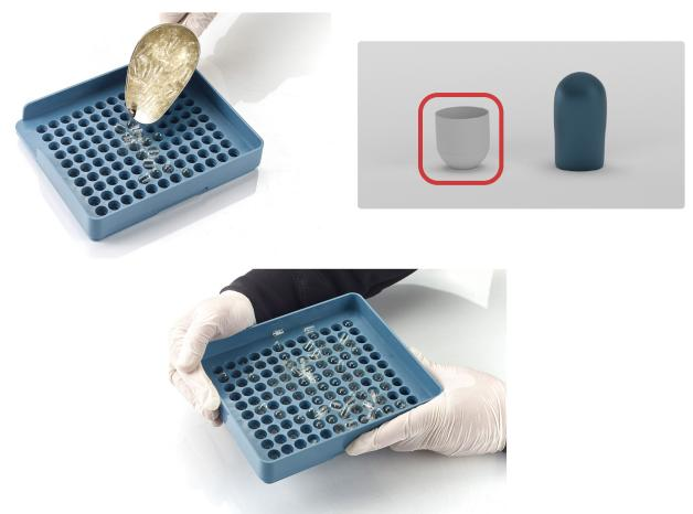
7. Remove the alignment plate from the cap plate and ensure that the capsule caps are in the correct position.
