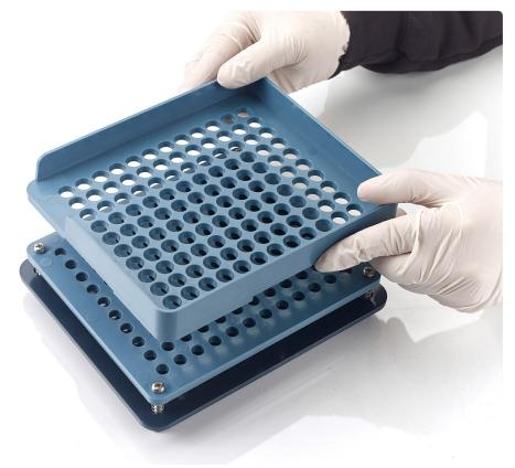
2. Pour the separated capsule bodies (120 count) on top of the alignment plate.
