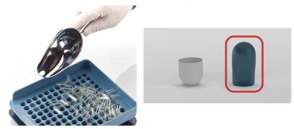
3. Shake the alignment plate and body plate so that the capsule bodies fall into the body plate.
