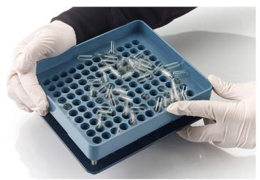
4. Remove the alignment plate and slightly press down the body plate to ensure that all the holes have capsule bodies and that they are positioned correctly.
