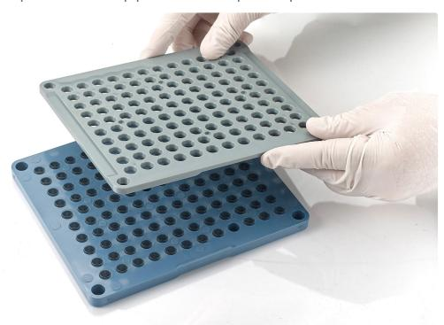
12. Turn over both the middle plate and cap plate 180 degrees and place them on the body plate.
