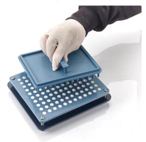
11. Insert the middle plate onto the cap plate with the capsule caps.
