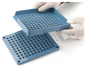
6. Pour the capsule caps (120 count) onto the alignment plate and shake the alignment plate and cap plate so that the capsule caps fall into the cap plate.
