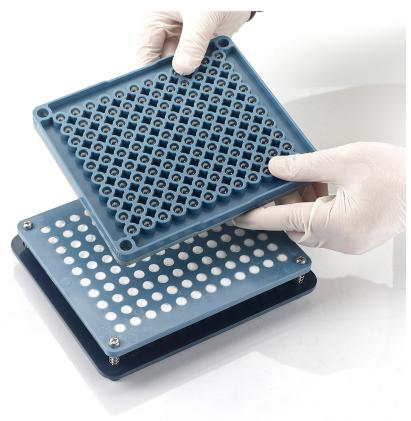
13. Push down all the plates together several times to seal the capsules.
