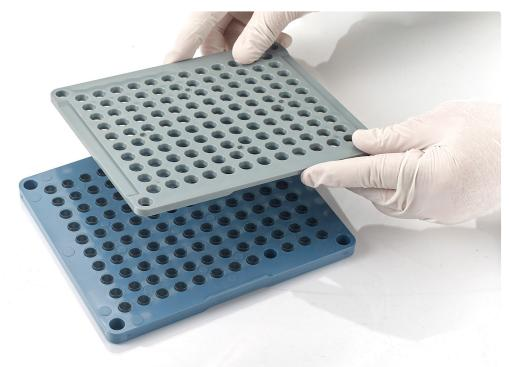
12. Turn over both the middle plate and cap plate 180 degrees and place them on the body plate.
