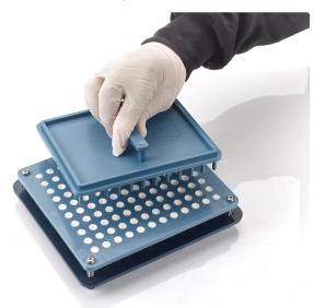
11. Insert the middle plate onto the cap plate with the capsule caps.
