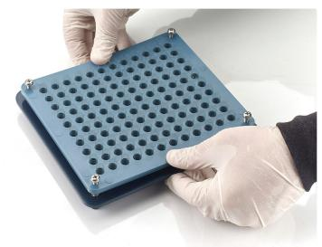
5. Place the alignment plate onto the cap plate.
