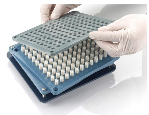
16. Remove the filled capsules from the cap plate.
