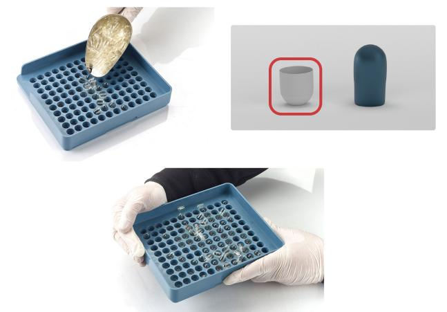
7. Remove the alignment plate from the cap plate and ensure that the capsule caps are in the correct position.
