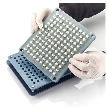
15. Separate the cap plate and middle plate.
