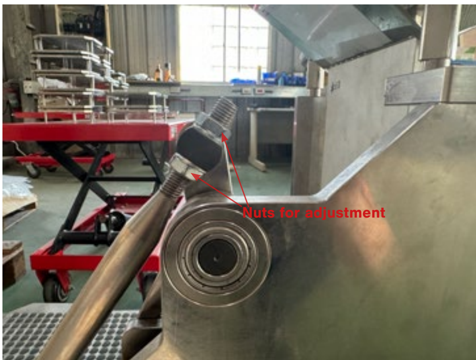
Fig-5 Adjust the nuts until the block gauge fits in the gap.
