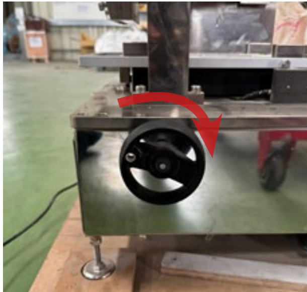
Fig-14 Rotate the handwheel clockwise.
