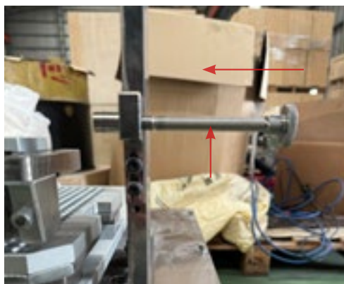
Fig-18 Push in the gate opening adjuster.
