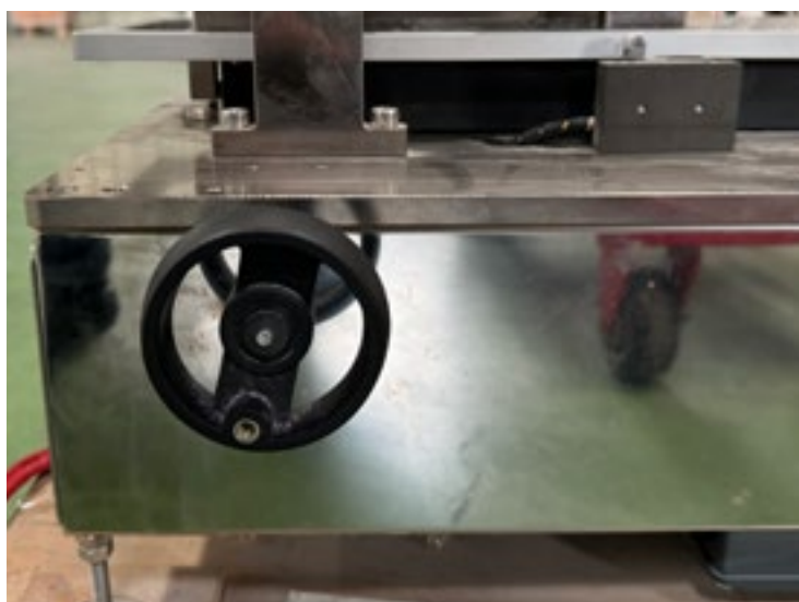
Fig-9 Insert the handwheel on the machine's right side.
