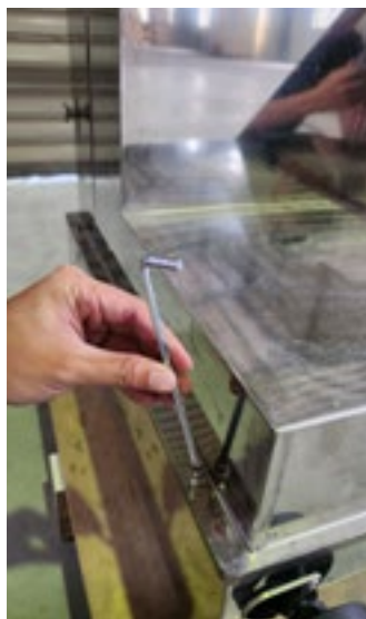
Fig-1.2 #5 Allen key used to remove the cover
