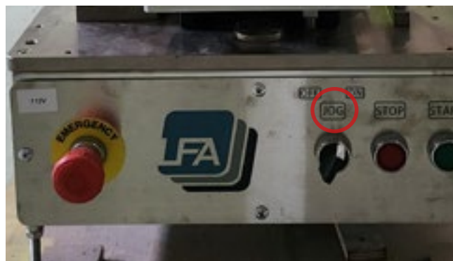
Fig-15 Switch the button to jog.
